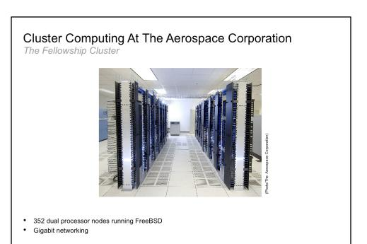
At Aerospace we have designed, built, and operated a FreeBSD HPC cluster since 2001. This picture shows the Fellowship cluster in it's current form with 352 dual processor nodes. In the process of building and running Fellowship we have ported a number of open source HPC tools to FreeBSD. In this talk I will discuss the process of porting them, issues we encountered, and a few pet peeves about application portability.
