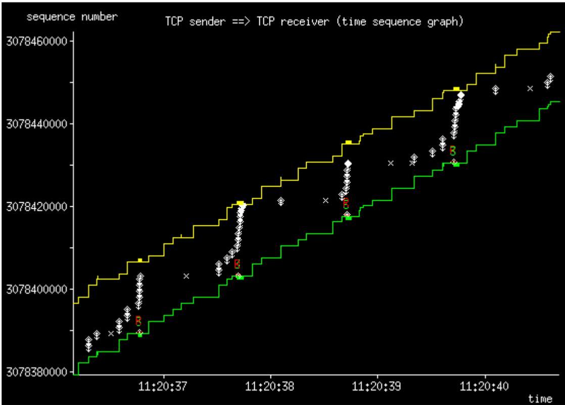
Figure 13: Blind flooding attack (time sequence graph)
