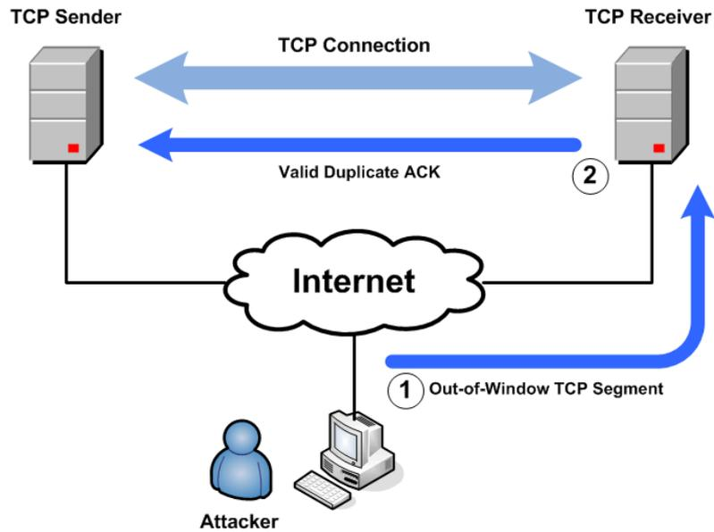
**Figure 10: Blind Dup-ACK forgery attack**
