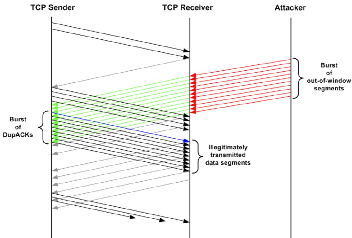
Figure 12: Blind flooding attack (time-line graph)
