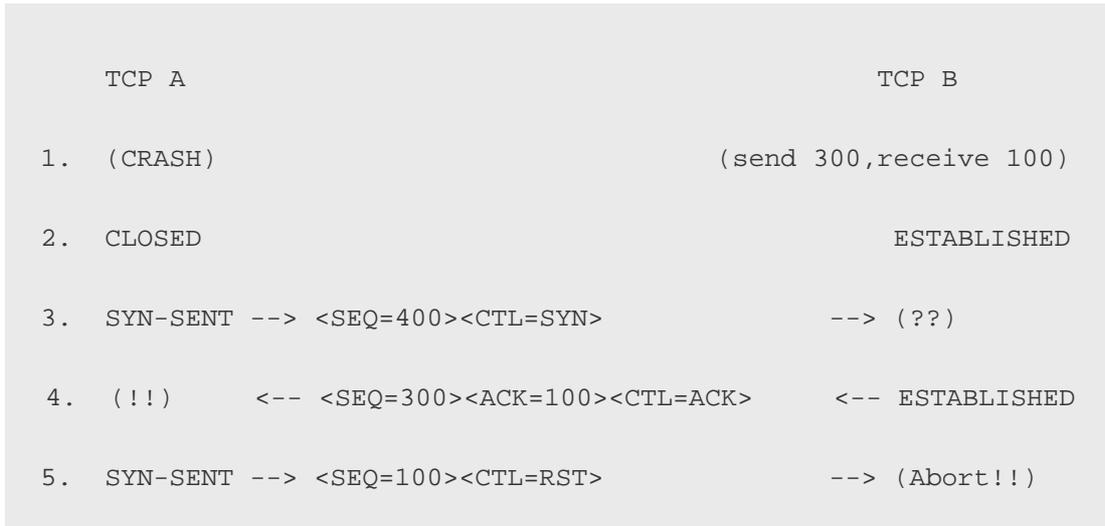
**Figure 17: Half-Open Connection Discovery**
