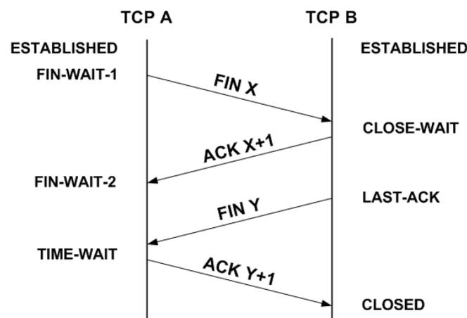
Figure 6: TCP connection-termination mechanism
