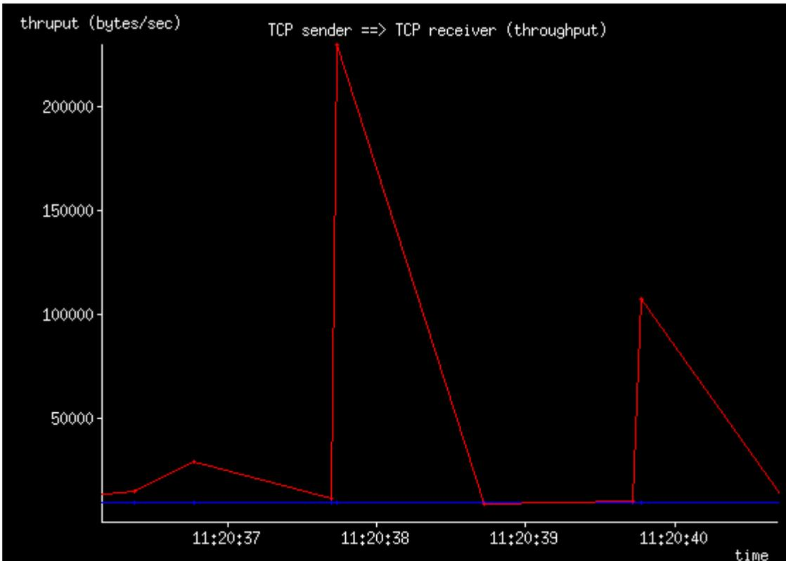
Figure 14: Blind flooding attack (averaged throughput graph)
