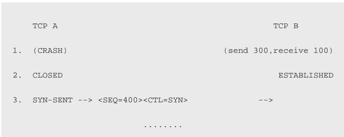
**Figure 18: Half-Open Connection Discovery with the proposed counter-measure**
