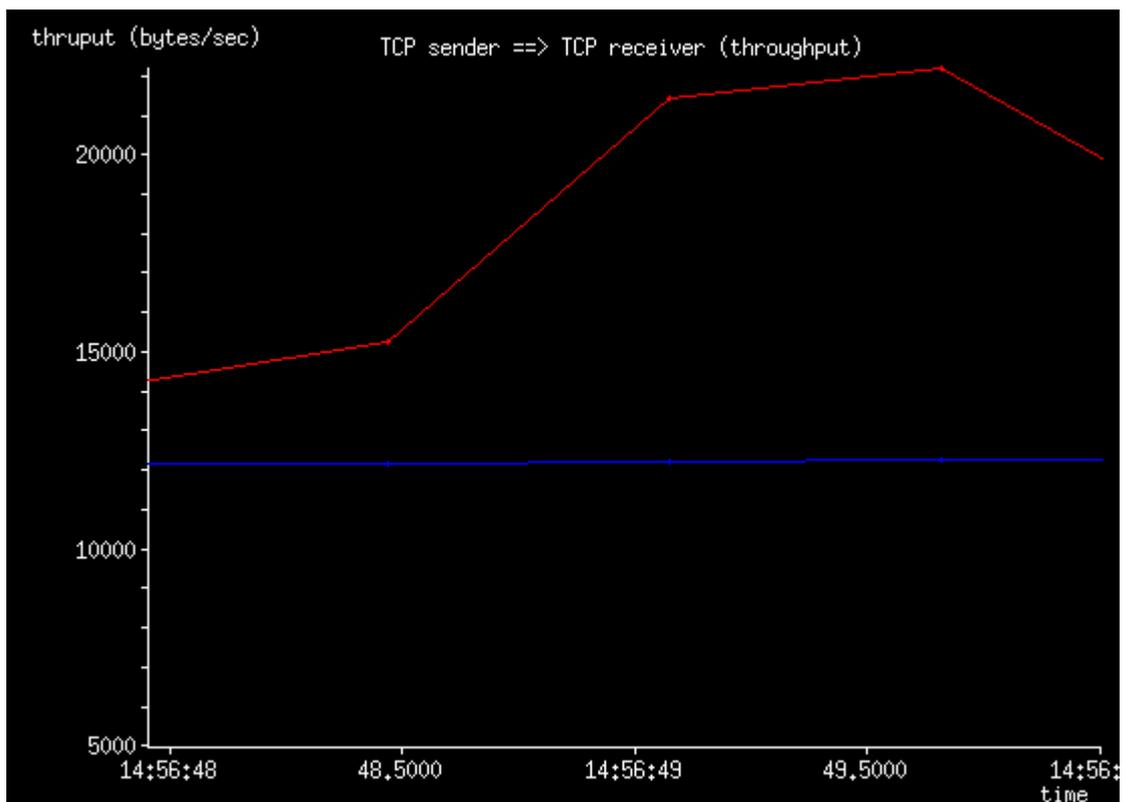
Figure 16: NewReno loss recovery (averaged throughput graph)
