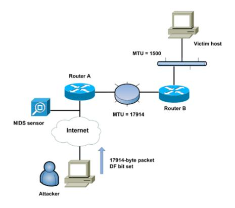
Figure 3: NIDS evasion by means of the Internet Protocol DF bit
