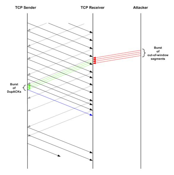
Figure 11: Blind throughput-reduction attack (time-line graph)
