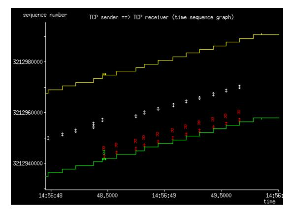
Figure 15: NewReno loss recovery (time-sequence graph)
