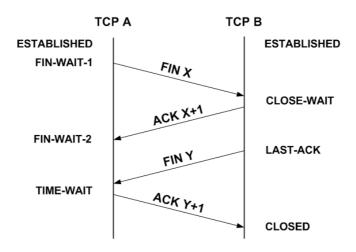
Figure 6: TCP connection-termination mechanism
