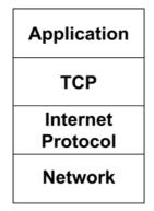
Figure 1: TCP in the DARPA reference model
