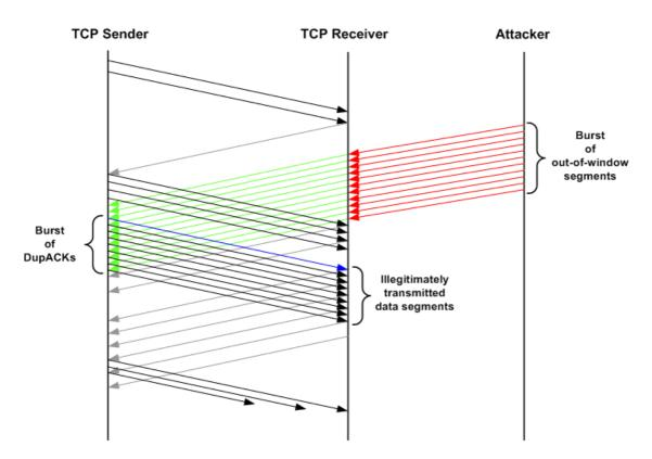
Figure 12: Blind flooding attack (time-line graph)
