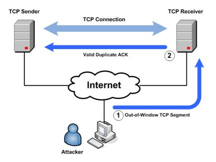
Figure 10: Blind Dup-ACK forgery attack
