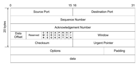
Figure 2: Transmission Control Protocol header format
