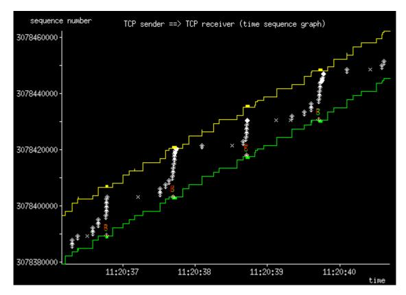
Figure 13: Blind flooding attack (time sequence graph)
