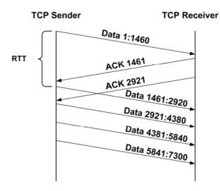
Figure 9: Optimistic ACKing attack
